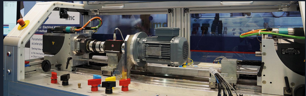
Turnkey test stand for electric motors produced by IMC Dataworks
